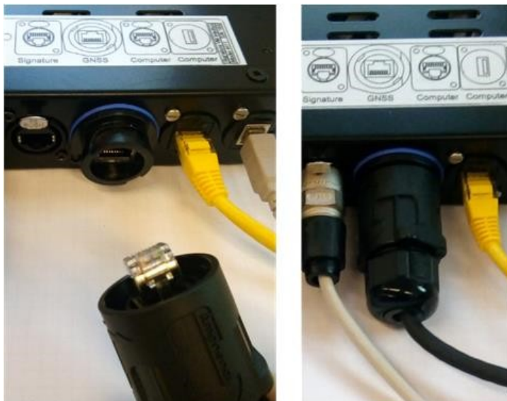
Figure 12: Connecting the GNSS to the interface
