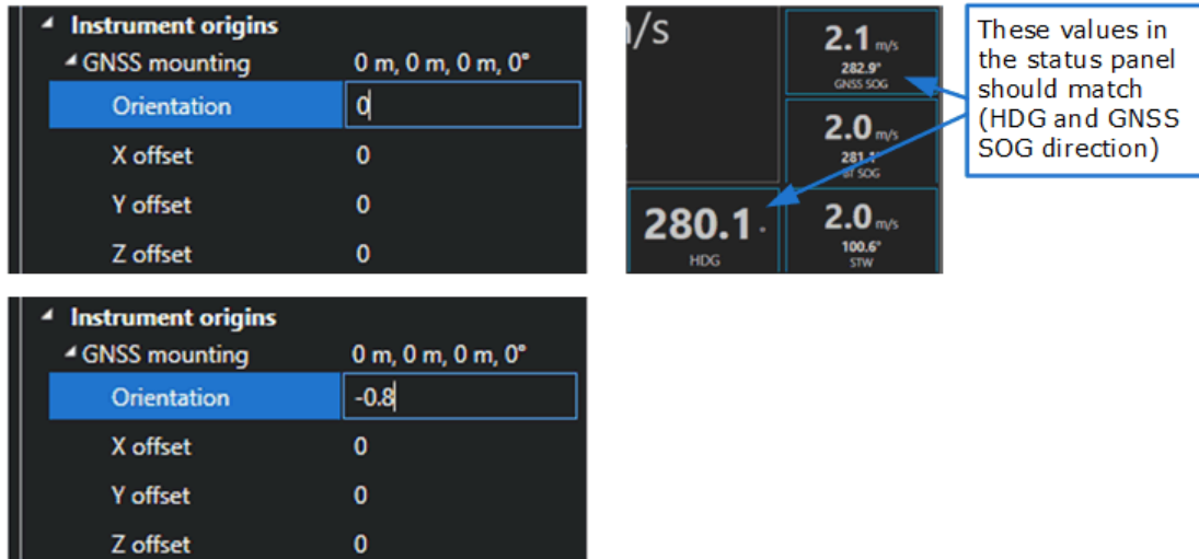
Figure 54: Adjusting GNSS orientation and settings
