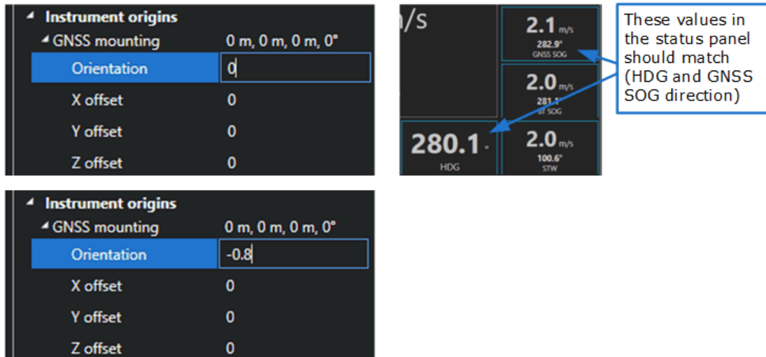
Figure 54: Adjusting GNSS orientation and settings
