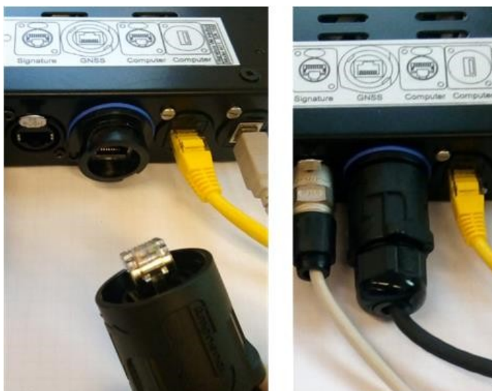
Figure 12: Connecting the GNSS to the interface
