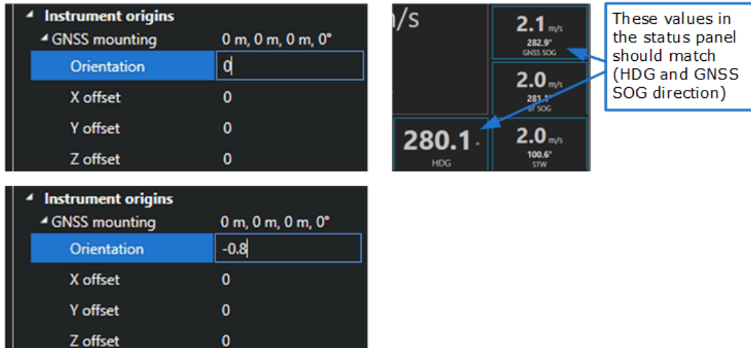
Figure 55: Adjusting GNSS orientation and settings
