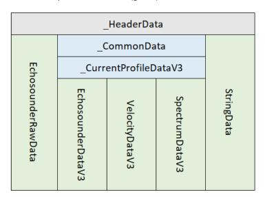
Figure: Showing how common data fields (gray for header and blue for other common's) the sensor data relate to the sensor specific data fields (green). Note that we use a leading underscore (\_) to emphasize that this is not a sensor data format but is common and used by two or more data formats.
