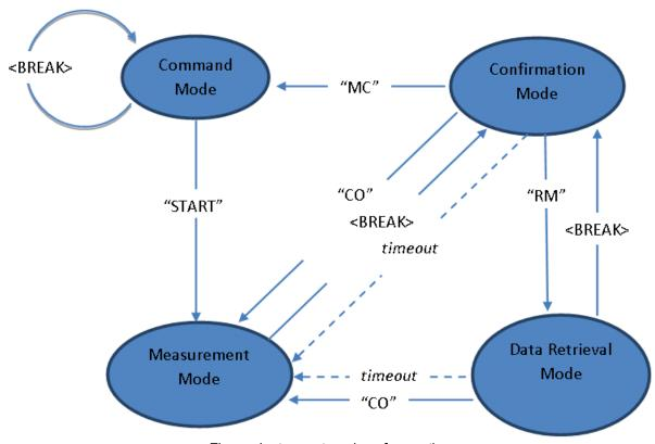
Figure: Instrument modes of operation
