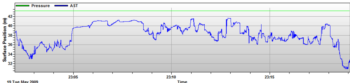
Figure 2: Example of time series of pressure and distance estimates. From this one can find the ice draft thickness.
