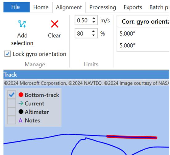
Figure 18: Correct VM-ADCP alignment
