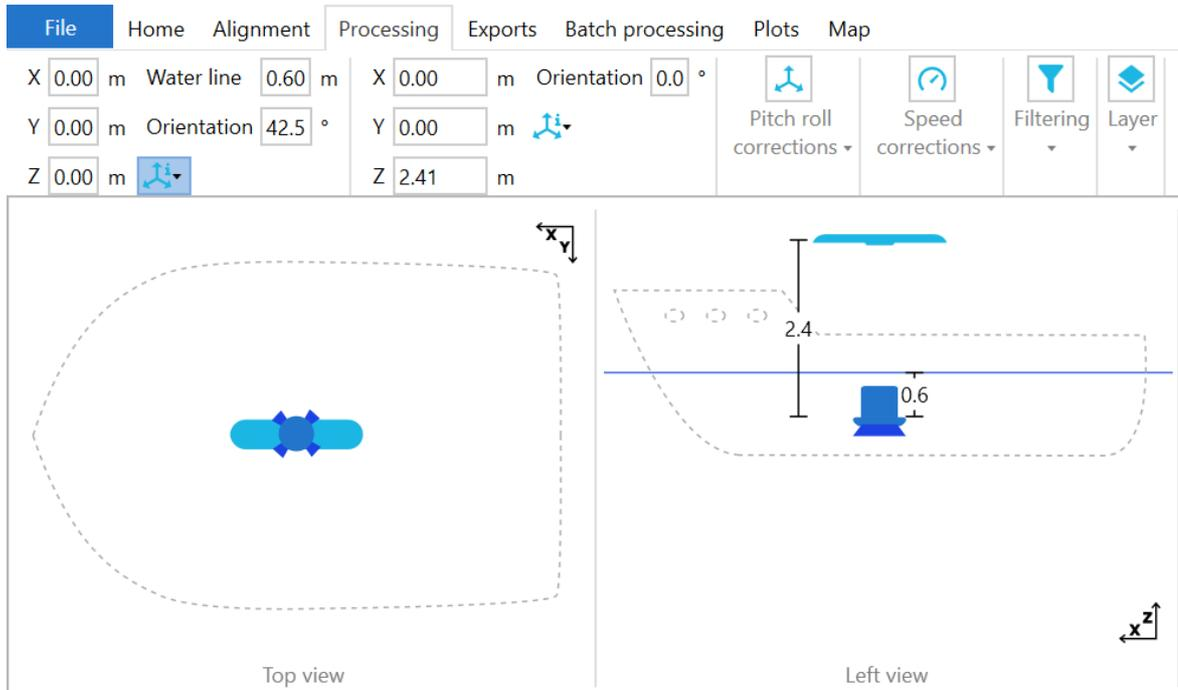
Figure 21: Offsets diagram
