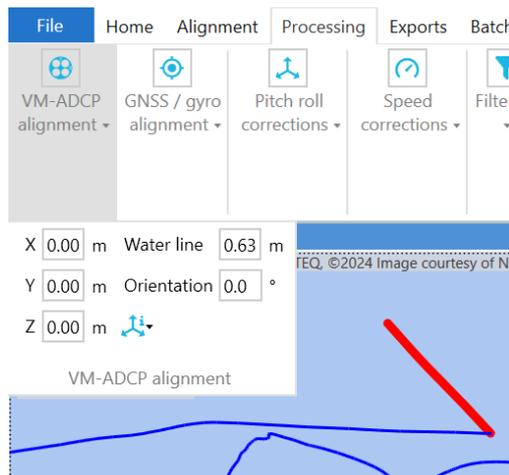
Figure 17: Incorrect VM-ADCP alignment
