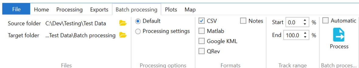
Figure 30: Batch processing menu
