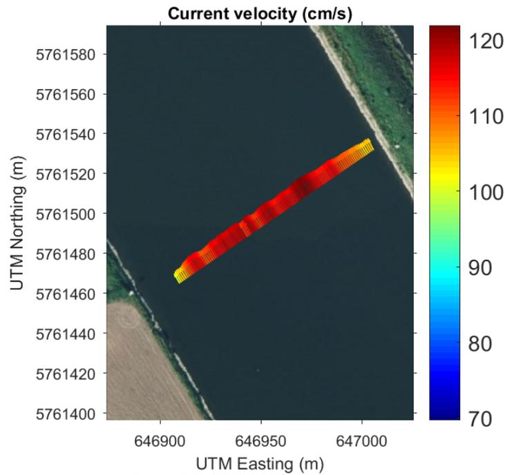
Figure 29: VMT track with current vectors
