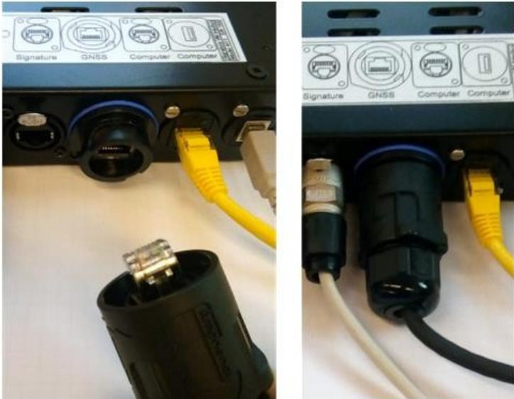
Figure 32: Connecting the GNSS to the Interface Box
