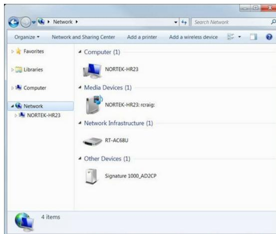
Double clicking on the instrument icon brings up the web page interface. Right clicking and selecting Properties gives the IP address and other instrument configuration information.
