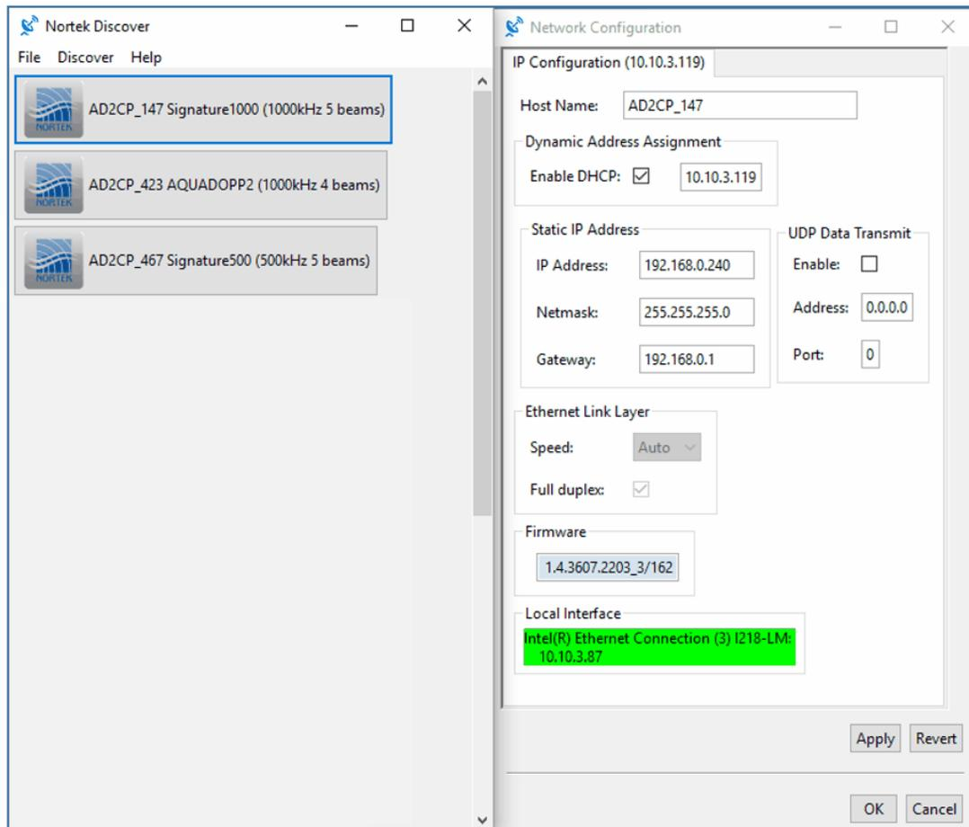
Once found, IP address information is displayed to facilitate a connection. Note: If the Local Interface is highlighted in red, it will not be possible to connect to the instrument because the IP configuration does not match that of the computer running the Discover protocol. The IP settings must be changed in the computer or the instrument to allow IP connectivity.
