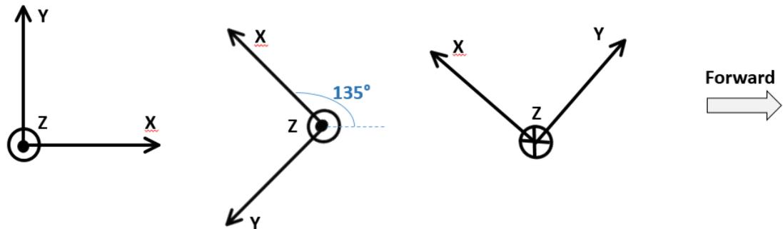
From left: Nortek DVL coordinate system, Legacy coordinate system and definition of "Forward" direction
