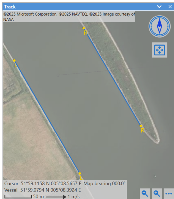
Figure 33: Marking the banks of the channel for discharge calculation
