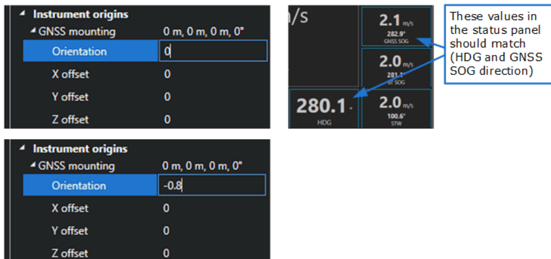
Figure 66: Adjusting GNSS orientation and settings
