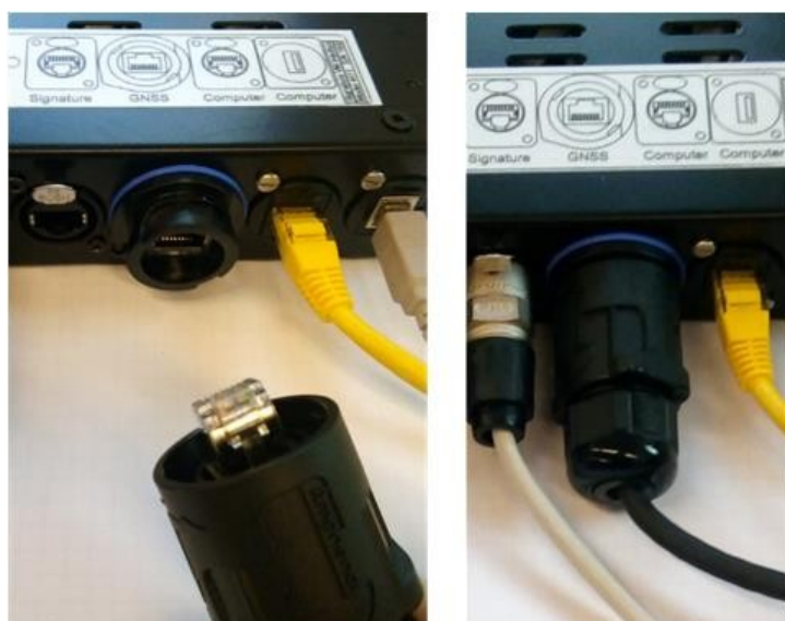
Figure 32: Connecting the GNSS to the Interface Box
