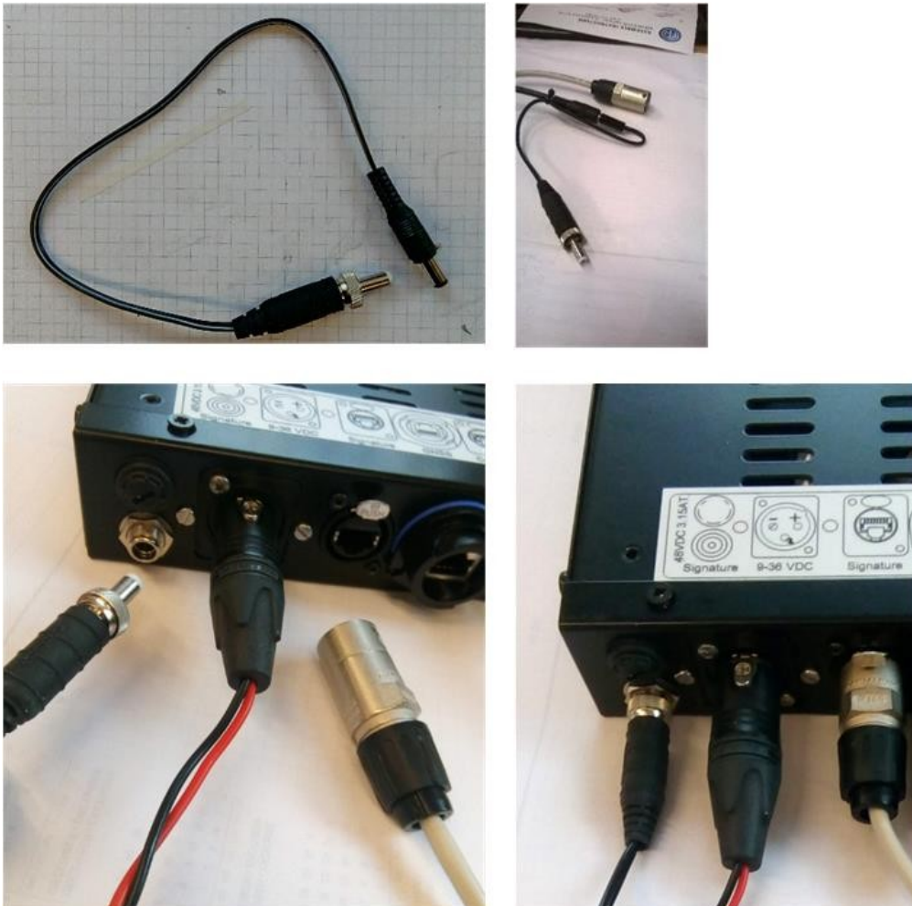
Figure 30: VM-ADCP power and data connection
