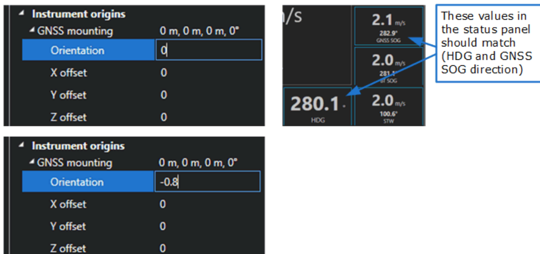
Figure 66: Adjusting GNSS orientation and settings
