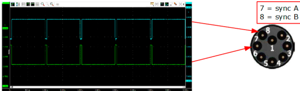
Figure 78: RS-485 triggering oscilloscope trace and connection pins
