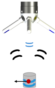
Figure 12: Transmit pulse pair (blue), a moving particle (red), and the reflected, Doppler shifted pulse (black).
