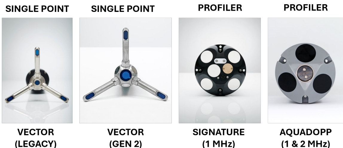
Figure 1: Instruments that operate with high resolution mode and rely on the pulse-coherent methodology.
