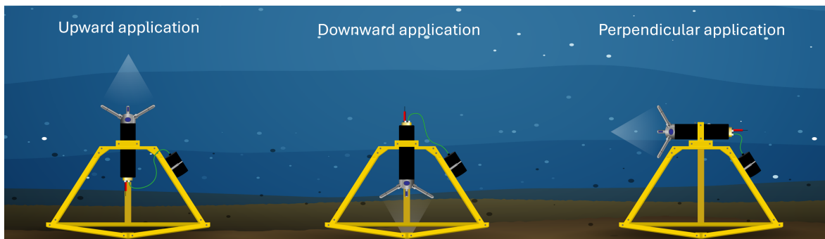
Figure 15: Examples of the Generation 2 Vector deployment configurations. The instrument is mounted on a bottom frame in various orientations, including upward-facing, downward-facing, and side-facing positions. Each setup is designed to optimize flow measurement depending on the surrounding environment and target observation zone.
