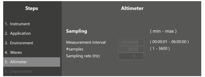
Figure 5. Configuration of an Alternating plan on Signature Deployment – step “5. Altimeter”
