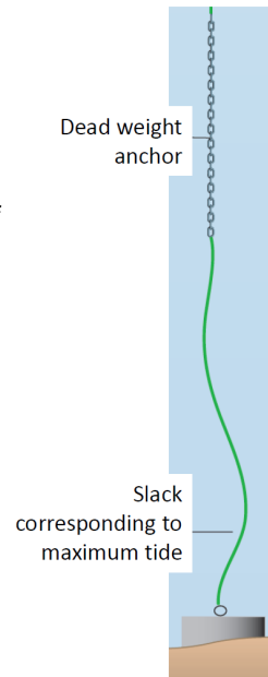
Figure 5: Illustration of the use of dead weight anchor
