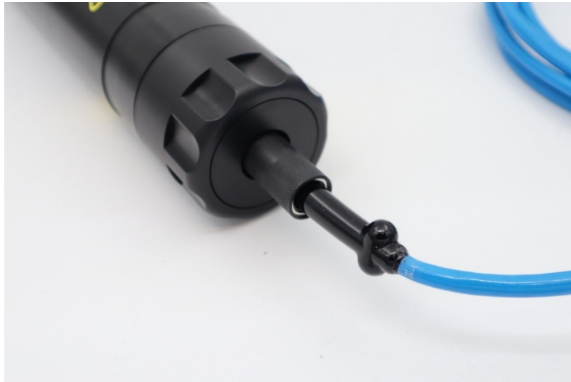
Figure 6. Close-up of the connector correctly attached to the instrument.
