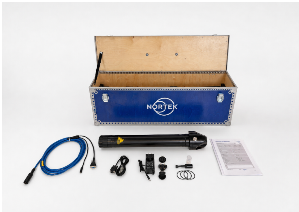
Figure 2. Overview of the Aquadopp Gen 2 case content.
