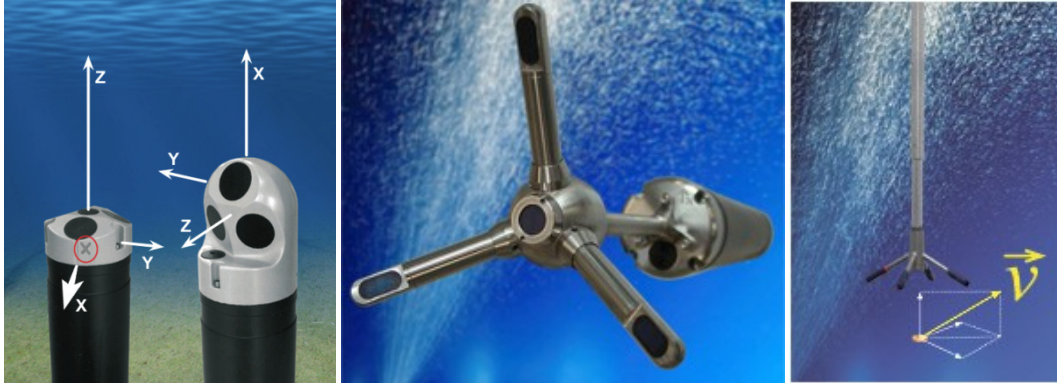
Figure 1. The three pulse coherent systems Nortek currently produces. (a) The Aquadopp/ HR Profiler and two standard head configurations. (b) The Vector with a fixed probe head. (c) The Vectrino with a fixed probe head.
