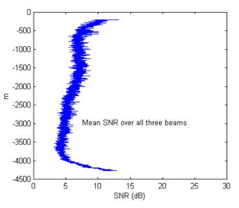
Fig. 6 – SNR data collected from the surface to the bottom in 4500 m of water in the Sargasso Sea. Data collected during transect from Woods Hole to Bermuda.
