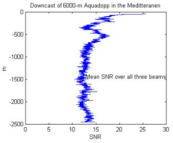
Fig. 5 – SNR data collected from the surface to the bottom in 2500 water depth in the Mediterranean.
