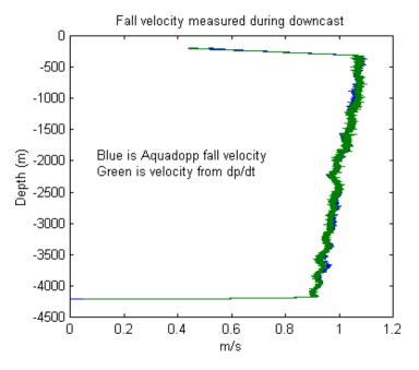
Figure 7 – Vertical velocity measured by the Aquadopp and calculated from the differentiated pressure data during the downcast
