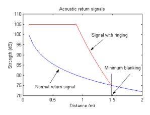
Fig. 2 – When the return the signal is weak, the acoustic ringing dominates the measured signal for some time after transmit. To avoid getting bad data, the ringing must be allowed to die out before sampling can start. Since the echo from the water gets weaker with time, the net effect of ringing is to reduce the sensitivity of the Doppler current meter. Ringing is specific instruments where the underwater housing is made from metal
