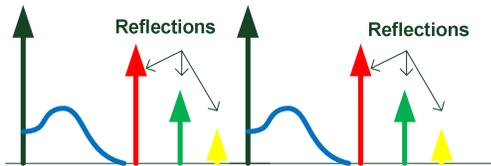
Figure 8. Ping rate chosen such that interference region dissipates before the next acoustic pulse is transmitted.
