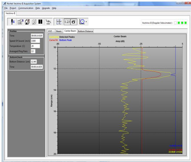
Figure 5. Bottom check data display
