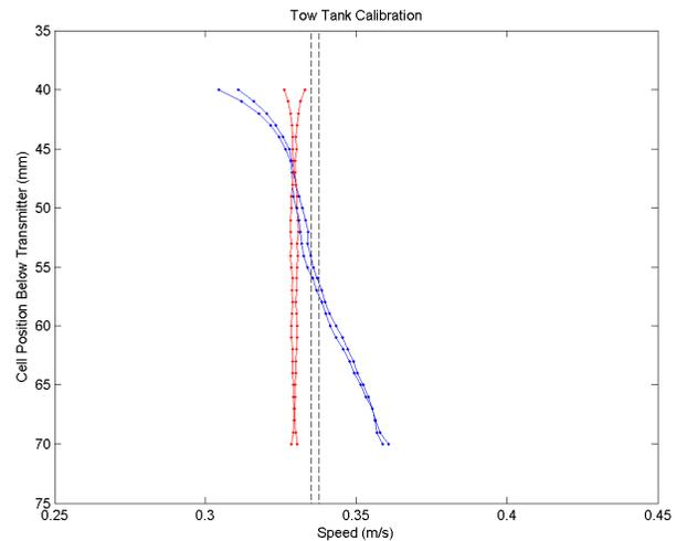
Figure 11. Tow tank data for Vectrino-II (two replicate tows). The blue line is a single matrix correction. The red line is a full profile correction.
