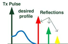
Figure 6. Single acoustic ping with multiple reflections from the initial transmit pulse occurring after the profiling region.
