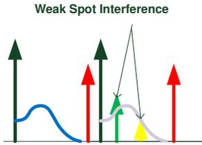
Figure 7. Reflections from the first acoustic pulse interfere with the sampling region of the second acoustic pulse
