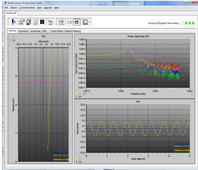
Figure 4. Real-time display of power spectra for velocity data
