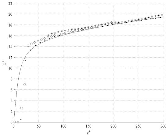
Figure 13. PIV (•) and Vectrino-II positioned at 70 mm (o) and 85 mm (\*) mean streamwise velocity profile plotted in wall coordinates. Spalart's DNS data is the solid line.
