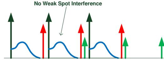
Figure 10. Ping interval selected such that sampling region occurs between reflections.
