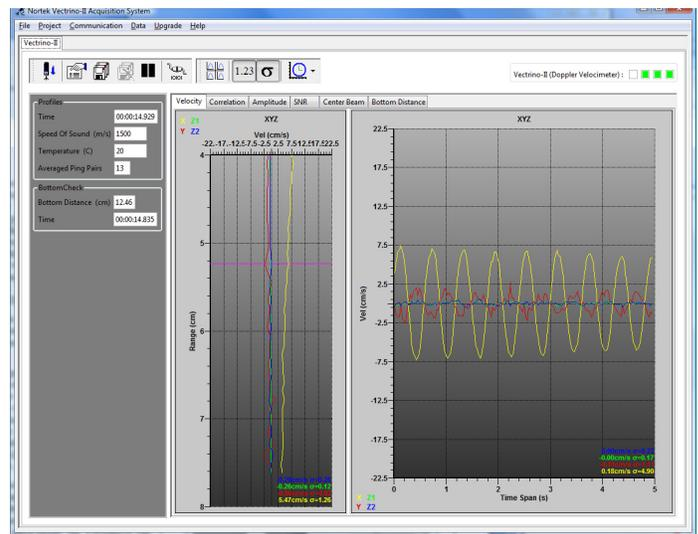
Figure 1. Basic display layout for acquisition software showing tabbed data displays combined with profile and time series plot views
