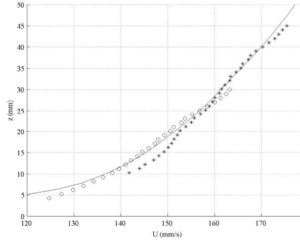
Figure 12. PIV (–) and Vectrino II positioned at 70 mm (o) and 85 mm (\*) mean stream-wise velocity profiles
