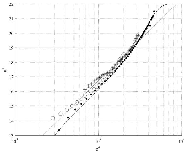
Figure 14. PIV (•) and Vectrino-II positioned at 70 mm (o) and 85 mm (\*) mean streamwise velocity profile plotted in semi-logarithmic wall coordinates. Spalart's DNS data is the dashed line while the Log Law (10) is the solid line.
