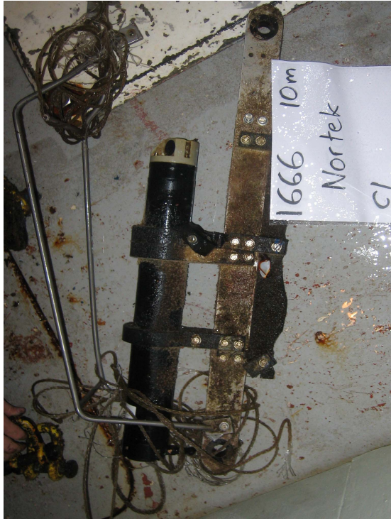
Figure 6. Climode 1 10m Aquadopp at recovery (Nov. 2006). Note the fishing gear, broken protecting bars, and broken vane on the load bar, opposite side from the instrument.
