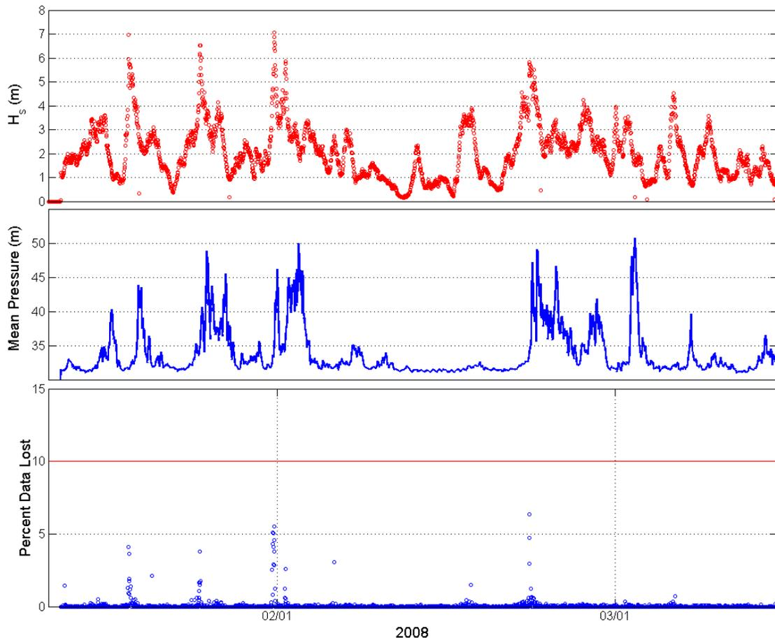
**Figure 6.** AST performance: (a) Significant wave height ( $H_s$ ), (b) Draw down depth of buoy, (c) Percentage of data loss resulting from bad AST detects, red line indicates threshold to discard AST time series in wave processing.
