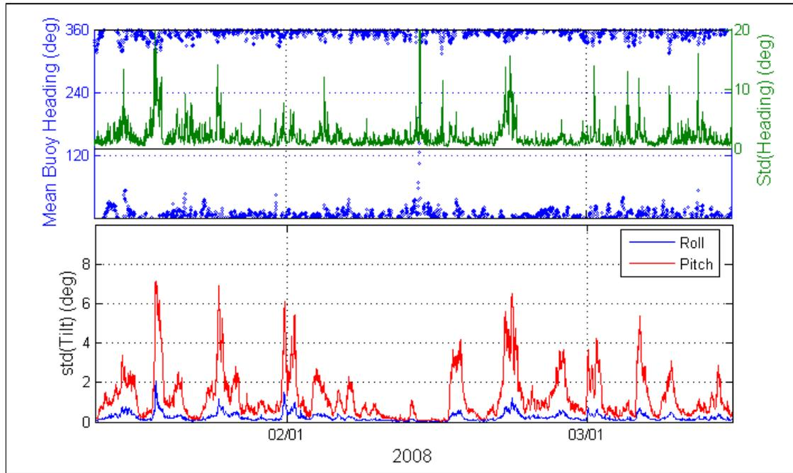
**Figure 4** Buoy Attitude during wave burst measurements. (a) Buoy mean heading (blue – axis left) and standard deviation of heading (green-axis right) during the burst. (b) Standard deviation of tilt.
