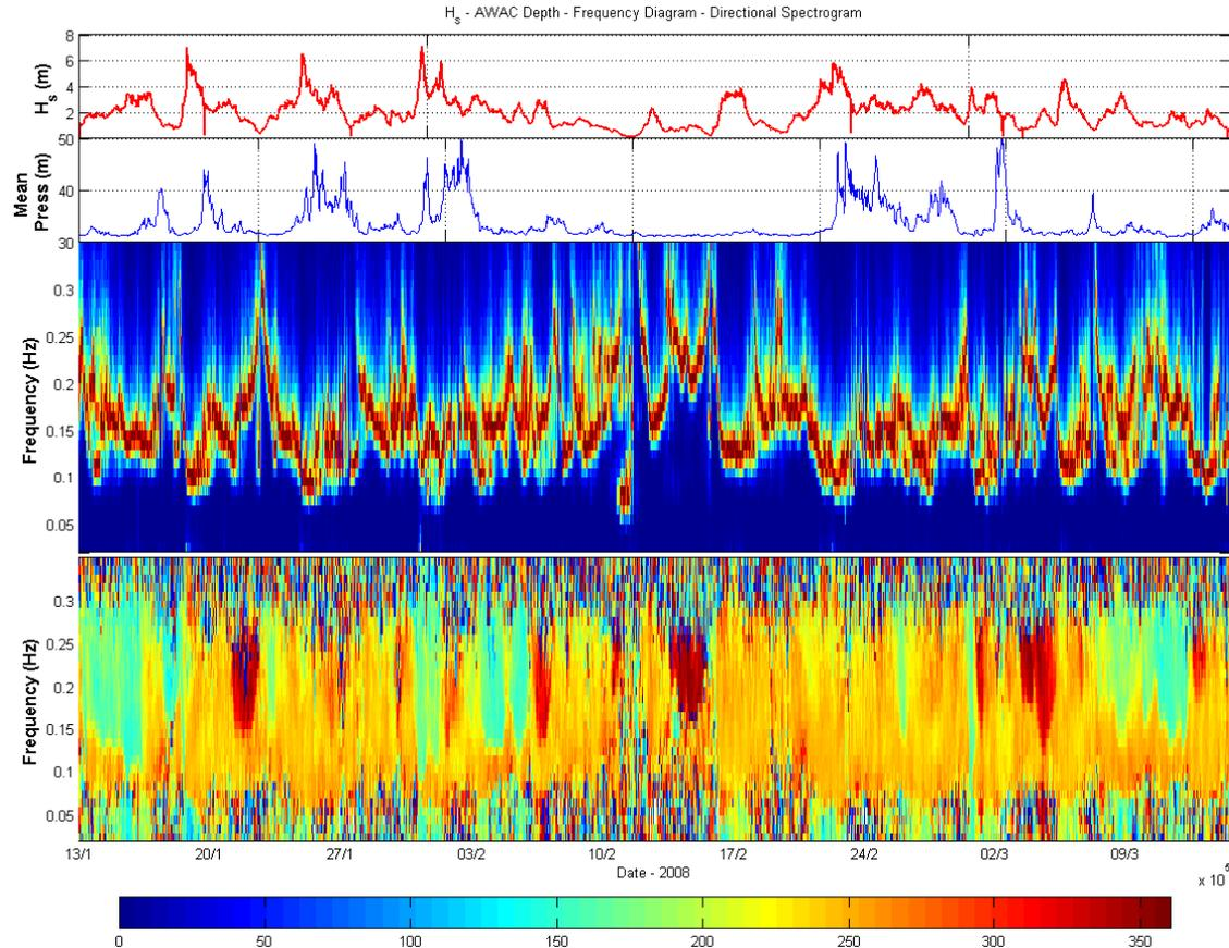
**Figure 8.** Summary plot of wave measurements, Lysekil. (a) Significant wave height, (b) AWAC depth, (c) Frequency diagram, (d) directional spectrogram.
