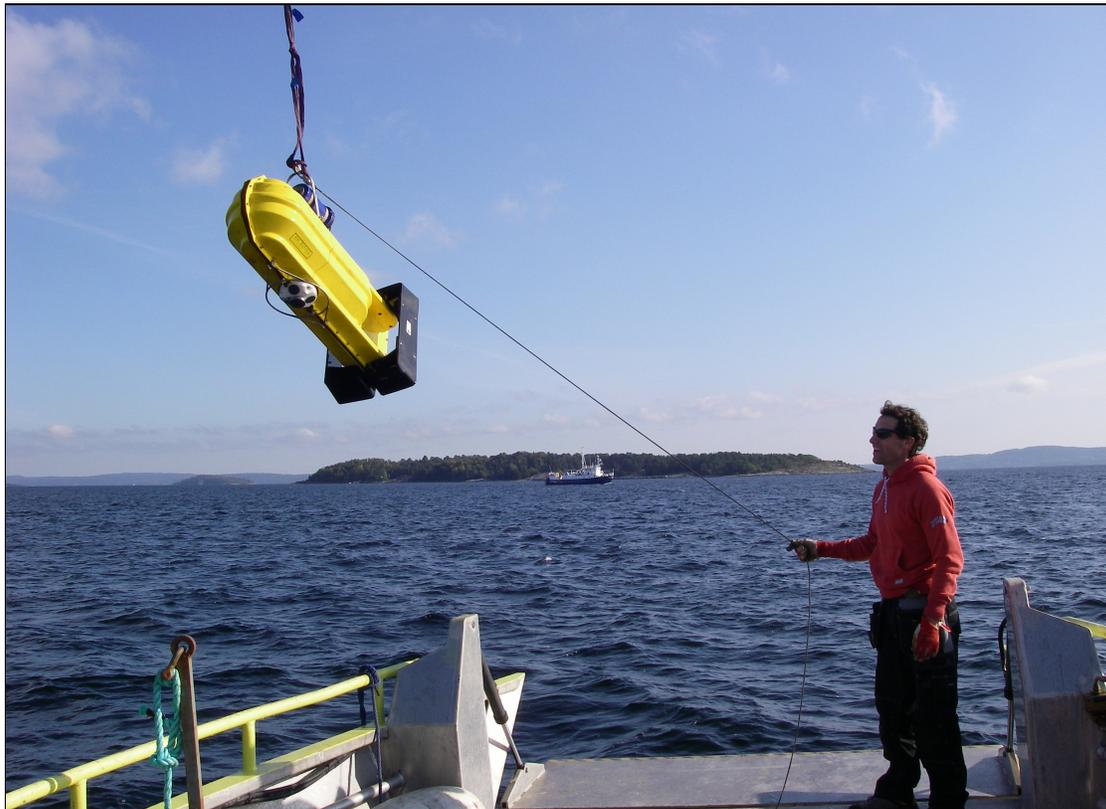
**Figure 1.** Deployment of a SUBS and AWAC (upside down) similar configuration to that used at Lysekil, Sweden.
