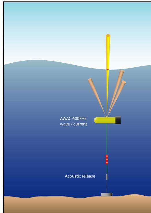
**Figure 3** Mooring configuration for 600 kHz AWAC mounted on a SUBS buoy. The four beams projecting away from the AWAC are the three slanted beams for velocity measures and a vertically oriented beam for Acoustic Surface Tracking (AST). The total depth at the Lysekil site was 120 meters and the mooring length was 90 meters.
