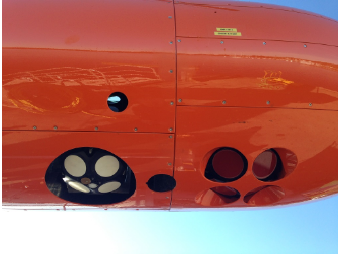
Fig. 4. Underneath HUGIN; the Nortek 500 kHz DVL to the left and the TRDI WHN 300 kHz DVL to the right.
