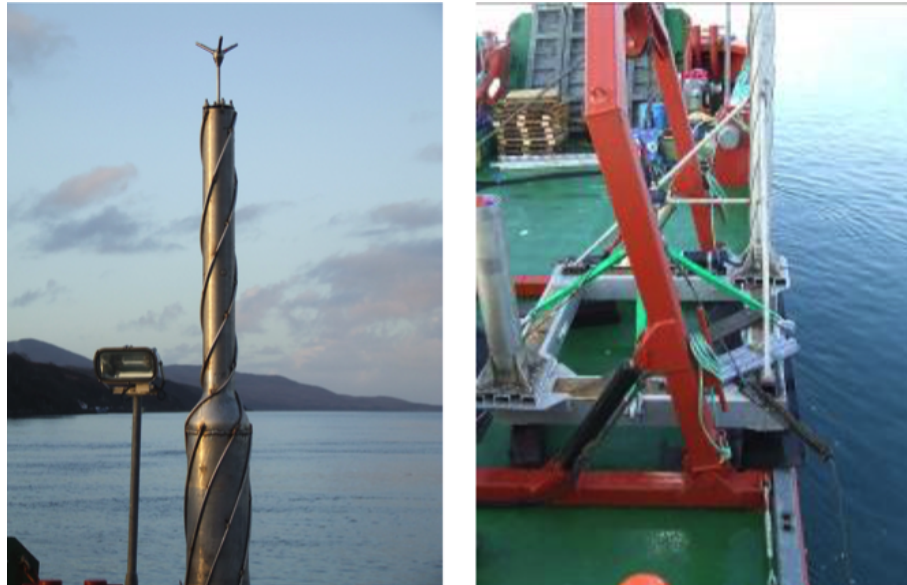
FIGURE 2.6 Measuring flow and turbulence at near-hub height; a 5-Tonne, 5 m tall frame was deployed to place a point current meter at 5 m above the bed (left photo; ADV at 5 m above bed). The large silver frame is shown during deployment on the right hand photo.
