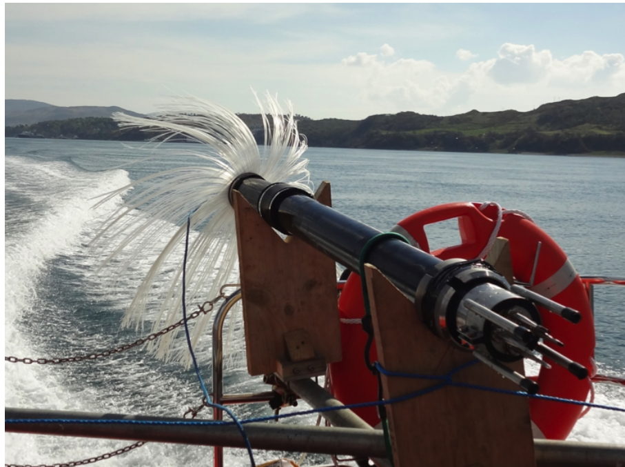
FIGURE 2.5 RSI Vertical Microstructure Profiler VMP200 with mounted sensors.
