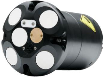
Fig. 5. The Signature1000 is a 5-beam ADCP with optional embedded AHRS, 1000 kHz frequency and maximum sampling rate of 16 Hz.
