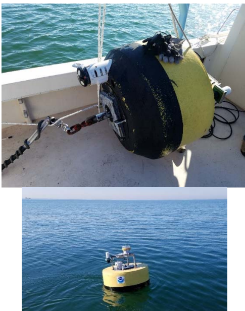
Fig. 6. The Signature1000 mounted on the 1.2 m diameter ionomer foam buoy, as seen during recovery (top) and during a calm day (bottom). Note the buoy was listing about 5^\circ , which was “desirable” to stress the limits of the test.
