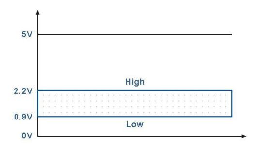
The output voltage levels for the SyncOut are:
