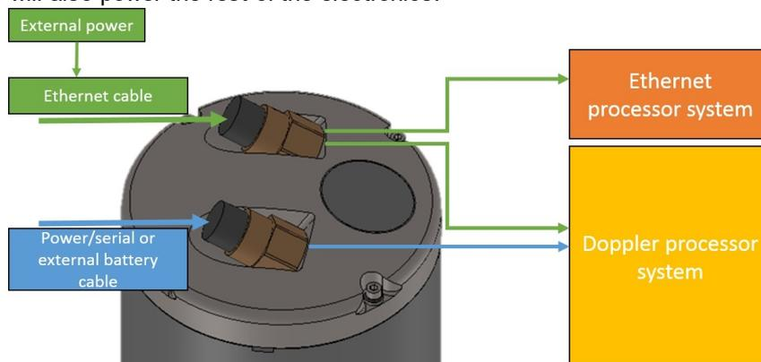
**Figure 3. Power distribution.** When the Ethernet cable is connected to the instrument, it will need to be powered from the power breakout cable. This will power both processor systems. If power is supplied through the Serial or external battery connector, the Ethernet processor is unavailable.
