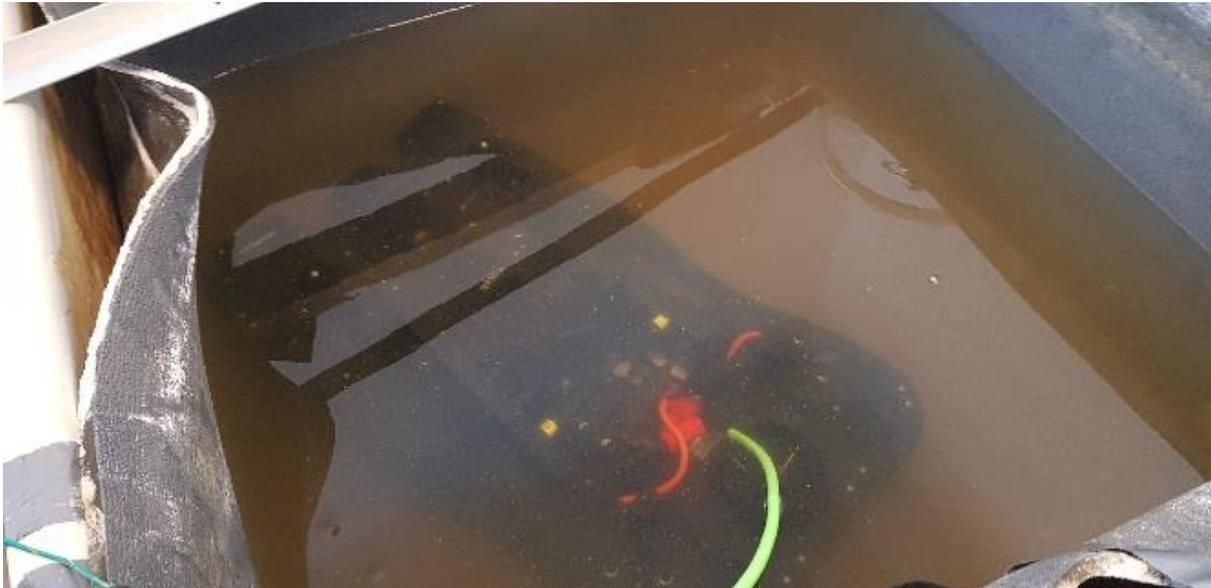
*Figure 1 Example of Faradays Cage in a saltwater tank.*
