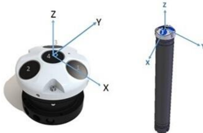
Figure: The AWAC and Aquadopp (symmetric head) XYZ coordinate systems and beam numbering as defined relative to the beams. Beam 1 point in the direction of positive X-axis; beam 1 of the AWAC and Aquadopp is marked with an X engraved on the housing.
