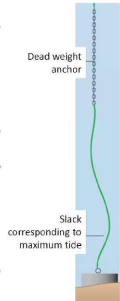
Figure: Illustration of use of dead weight anchor
