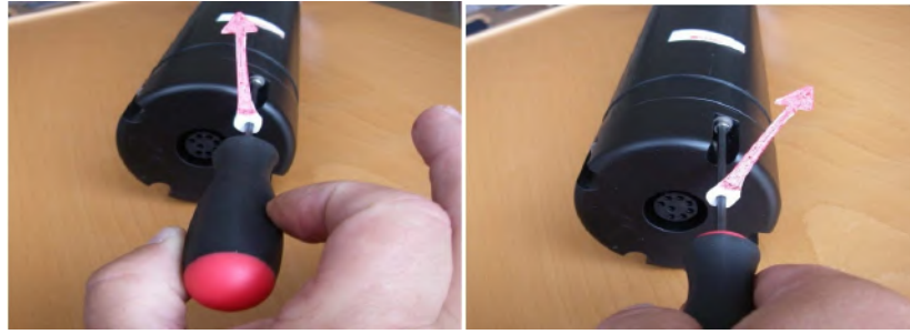
Figure: a) "Two-fingers" tightening of screws. Indicator arrow shows position before final tightening. b) Final tightening 30-45 degrees from "two-fingers" tightening.
