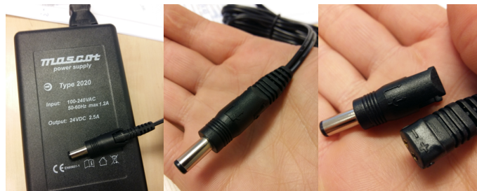
Figure 22. Make sure the plug on the power supply is correctly fitted if it has been disconnected earlier
